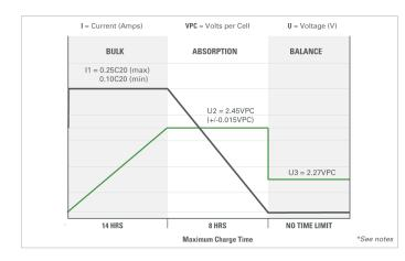
Due to self-discharge characteristics of lead-acid battery technologies, batteries should be top charged within 6 months of storage to ensure optimum performance, prevent sulphation and permanent capacity loss.
